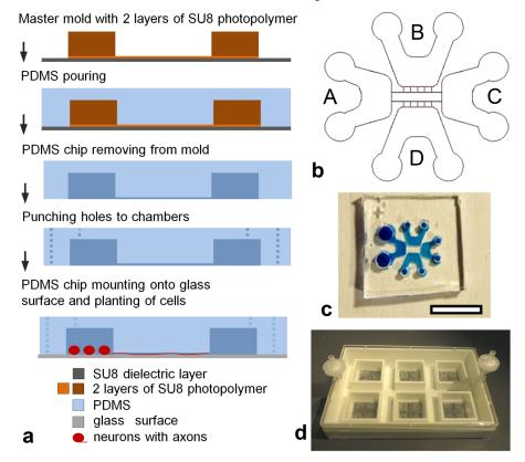
*Fig 1. Microfluidic chips a.* Microfluidic chip fabrication steps. b. Microfluidic chip design. c. Microfluidic chip combined with a cover glass. Scale 5mm. d. Design of the plate with the chips.
