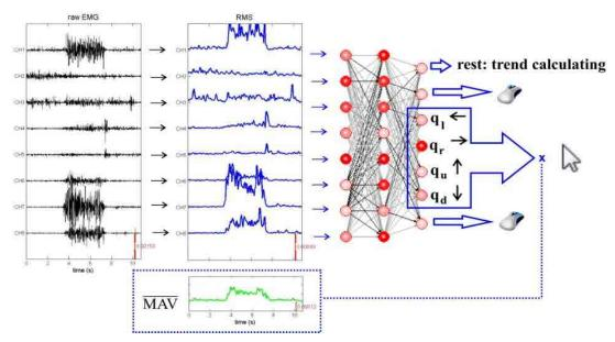
**Fig.1**. Information flux in the MyoCursor system. Raw sEMG activity is mapped into cursor movements and mouse clicks in Windows OS. First RMS and MAV activity is evaluated. RMS pattern is fed into the input layer of an artificial neural network with one hidden layer. The network output from seven neurons provides two commands for mouse-like clicking and four commands for cursor movements. These are multiplied by the MAV to gain the cursor speed
