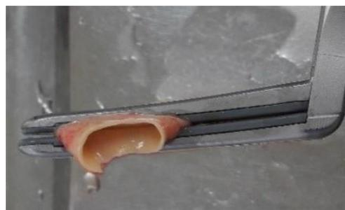
**Fig. 4.** Scheme of fixing the walls of the aircraft in the branches with their transverse clamping
