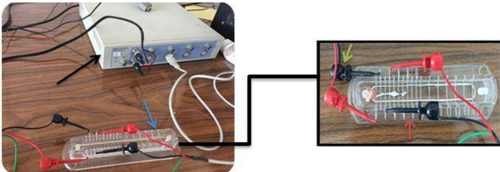
**Fig. 1.** A power lab device (black arrow) with stimulating and recording electrodes (green and brown arrows, respectively) connected to the wires of the nerve chamber (blue arrow)
