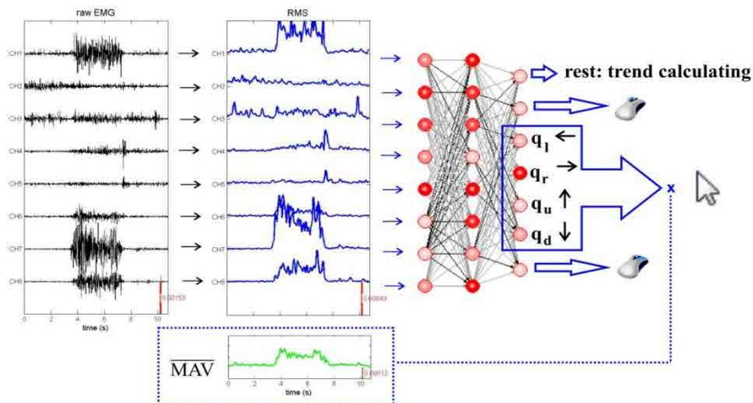
**Fig.1.** Information flux in the MyoCursor system. Raw sEMG activity is mapped into cursor movements and mouse clicks in Windows OS. First RMS and MAV activity is evaluated. RMS pattern is fed into the input layer of an artificial neural network with one hidden layer. The network output from seven neurons provides two commands for mouse-like clicking and four commands for cursor movements. These are multiplied by the MAV to gain the cursor speed
