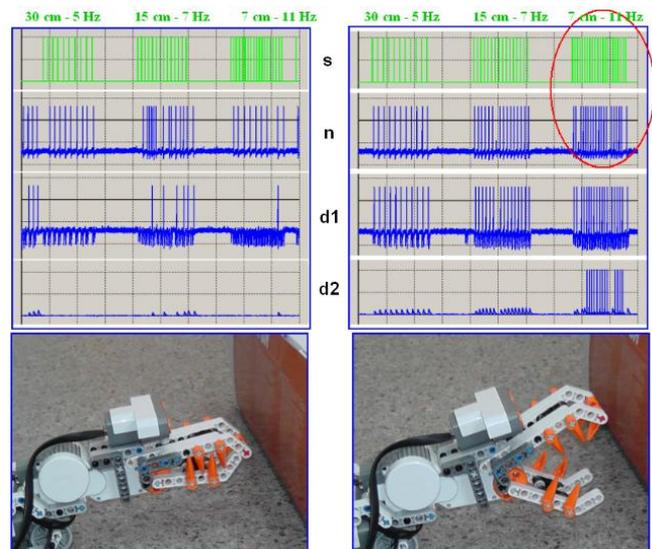
Fig. 1. “Eating” behaviour based on synchronization phenomenon in the animat. Left and right columns correspond to before and after learning, respectively. The output from the ultrasonic sensor (s) provokes synchronization (red circled) of neurons in the main network (n is a representative neuron). This in turn leads to activation of the phase filter neuron (d1) and later of the frequency filter neuron (d2) and the animat opens the jaws.
